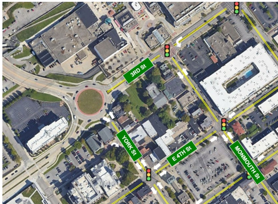
Figure ES-4: Two-Way Conversion of York Street and Monmouth Street with northbound York Street connection to roundabout
